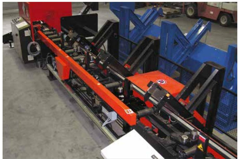
The transport and handling systems, depending on the chosen model, are suitable for loading and separation of bar stock up to a diameter of 140 mm and a bar length of 12 m. This equipment is highlighted by robust, low-maintenance design and highly suitable for operation under tough operating conditions, for example in forging shops.
